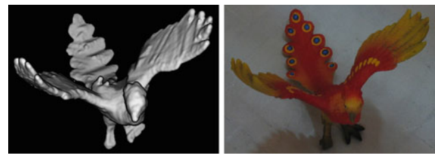
Fig. 5 Intensity-coded backprojection area element \mathcal{J}_i^\pi and corresponding input image. Some errors in the input geometry are clearly visible—no good texture can be expected in those regions
